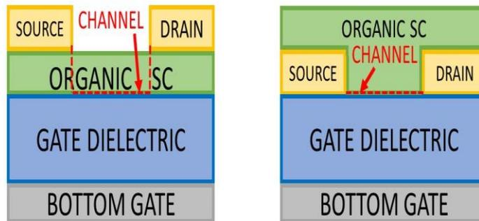
a) Staggered Architecture: Top-contact Bottom-Gate b) Coplanar Architecture: Bottom-contact Bottom-gate
